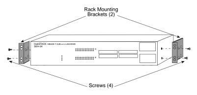
Figure 3-4. Installing the Rack Mount Brackets
